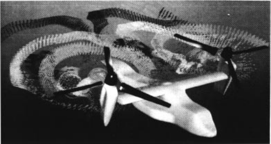
Figure 20 Streaklines for the V-22 Tiltrotor operating in the helicopter mode. From Meakin (1993).
