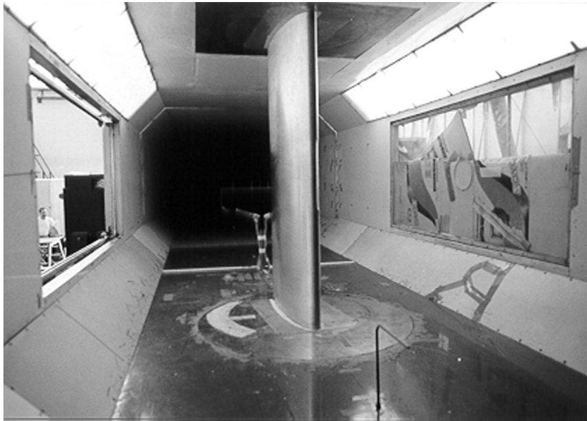
Fig. 5. Airfoil model installed in the test section.
